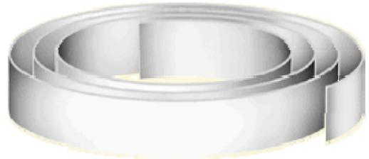
The finished cylinder should fit snug on the scope yet slide easily on and off. The fit is very important – too tight and you can't get the filter on and off without damaging it – too loose and an accidental bump or a gust of wind could knock the filter off.
