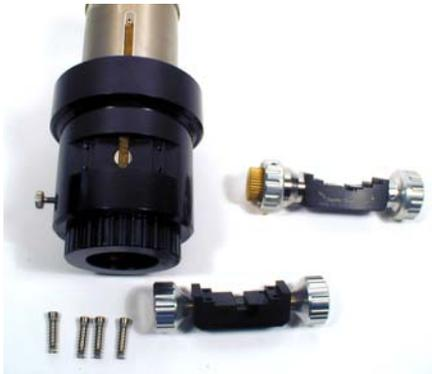
With a 3/32" hex wrench, remove the 4 screws holding the standard pinion block and knob assembly from the focuser body.
