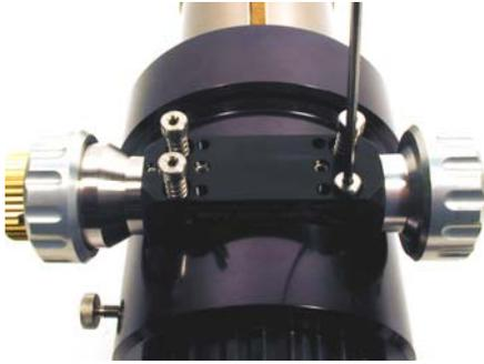
Place the new Feather Touch block onto the focuser body as shown for right hand operation, or reverse it for left handed operation. Tighten down the 4 shoulder bolts with the springs using a 3/32" hex key.
