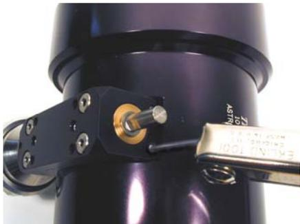
Gently tighten the two small setscrews, with a 1/16" hex key so that they just touch the mating focuser body. Do not over tighten these screws. Re-attach the knob, making sure that the washer is still under the knob on the pinion shaft.
