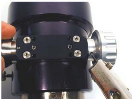
Loosen the knob opposite the reduction gear with a 5/64" (Traveler and 2.7" Focuser) or 1/16" (4" Focuser) hex key and remove it from the pinion.
