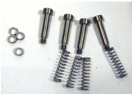
If the pinion block shoulder screws have spacers under the springs (some do, some don't), remove the springs and spacers. Keep the orientation of the springs the same as they were (do not turn them end for end).
