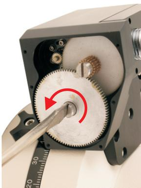
Remove the cover to expose the clustered spur gears beneath. The worm's spur is hidden underneath the large spur gear that is on top of the cluster. This top cluster gear must be removed.
