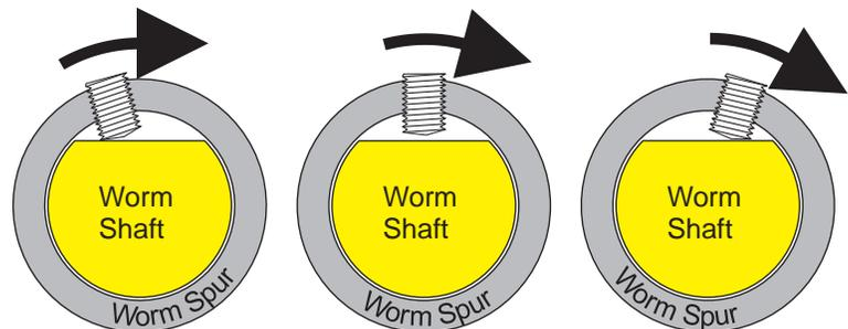
Loose Spur Gear Set Screw Causing Slop in Gear Train. Spur Gear Turns Without Turning Worm Gear.
