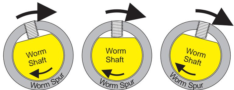
Correct - Tight Set Screw Centered on the Flat Spot on the Worm Shaft Causes Worm to Turn with Spur Gear
